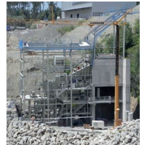
MASTER Primary crushing plant, limestone, 600t/h, HAVER F-CLASS, HAVER push feeder, impact crusher
