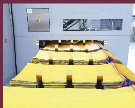
tailor-made: empty bag magazine (maximum capacity: 600 bags)
