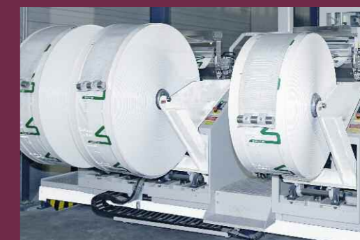
time-saving: automatic reel changer – in variants for 2 or 3 reels – for reduced standstill times in case of film reel changes
