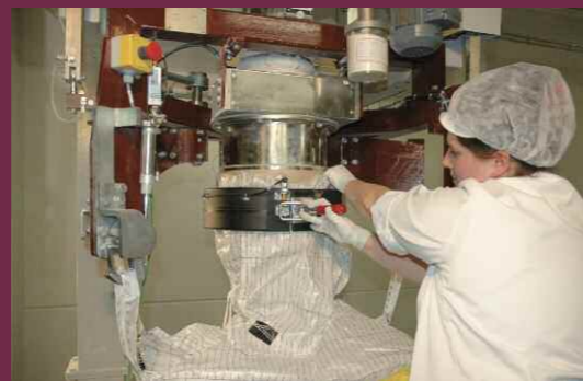
fixing of the filling spout – with inflatable sleeve for dust-tight big bag sealing during filling
