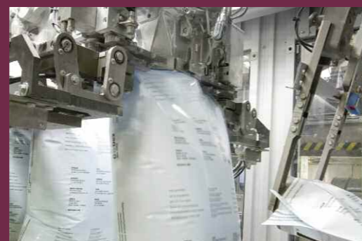
Hygienically filled: Product filling by the dust-tight special powder spout with integrated residual air de-aeration
